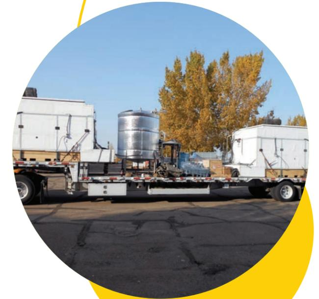
Figure 1: A dry anaerobic digestion pilot plant ready for transportation to Mexico.
