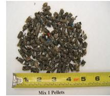
*Pellets produced from residual wastes from the City’s composting and recycling facilities*
